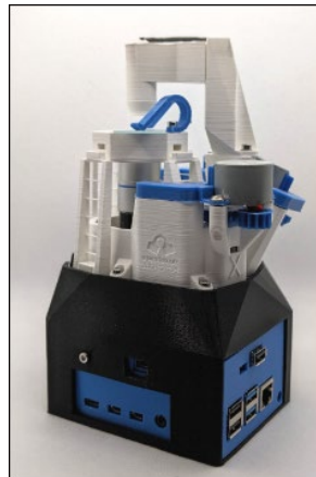
Figure 4. An open-source 3D printed microscope.
